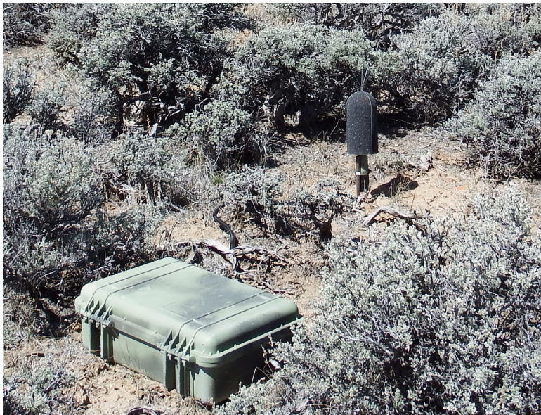
FIGURE 2. Typical deployment of equipment for measuring sound levels, showing case holding sound-level meter, digital recorder, and batteries, and microphone (with foam windscreen and spike to discourage birds from perching on it) 0.3 m above ground in sagebrush >0.3 m high.
